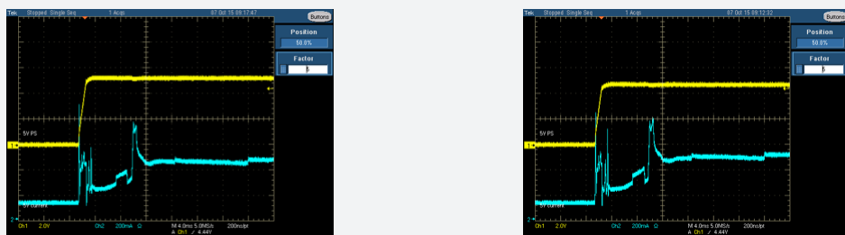
Figure 1. Typical Cold (Left Figure) and Hot Voltage/In-Rush Plots
