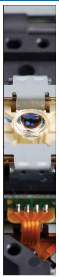
Detectors consist of a photodiode, amplifier, voltage regulator, Schmitt trigger, and output stage with a 10 kOhm pull-up resistor, open collector, or totem-pole output. IR LED sensors facing Optoschmitt detector in plastic molded housing – switching occurs when opaque object passes between emitter and detector. Digital output used for presence/ absence, motion sensing and encoding.
