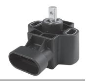
Round and round the globe, it's Honeywell. So trust Honeywell Sensing and Control (S&C) for your Hall-effect rotary position sensor needs. These sensors vary output voltage or current in response to changes in a magnetic field — using a magnetically biased Hall-effect integrated circuit (IC) to sense rotary movement of the actuator shaft. The rotation of the shaft changes the IC's position to the magnets, and then detects the change in
