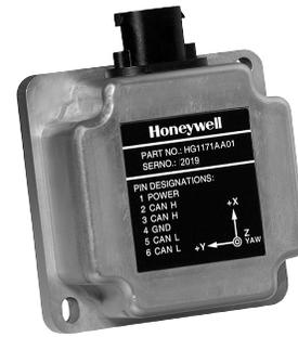
**Six degrees of freedom.** Provides three-dimensional motion sensing by detecting changes in rotation and how fast the equipment is moving. Precisely measures the equipment's dynamic motion and orientation, enhancing accuracy, and increasing safety, productivity, stability, and operational capability. A temperature sensor in each rotational rate sensor
